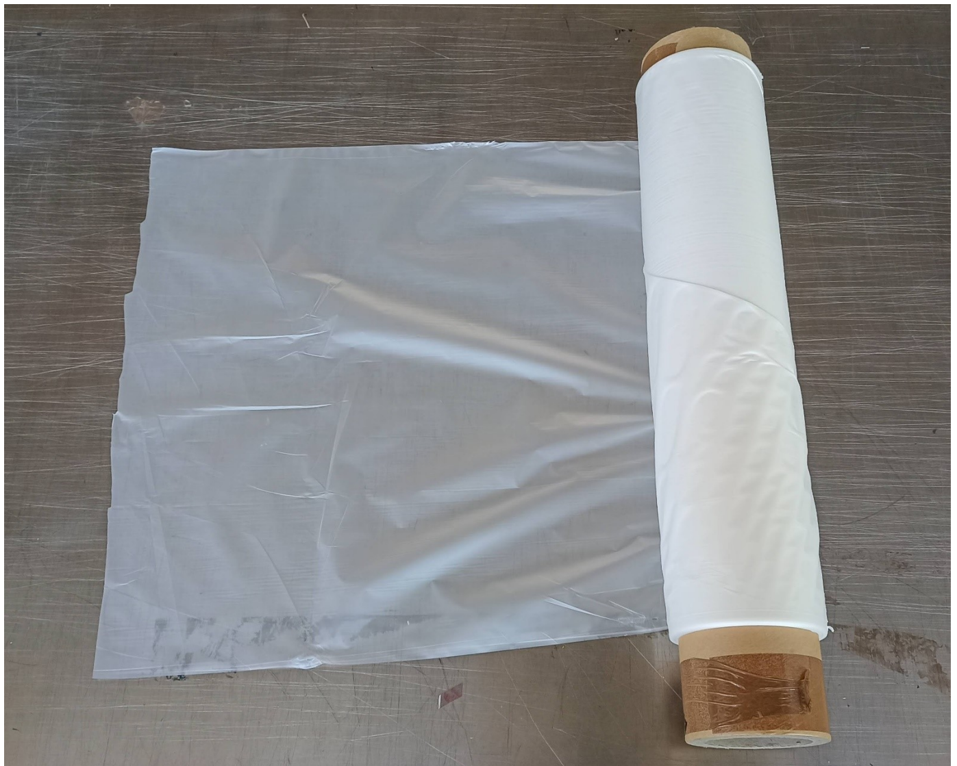
Film blowing of biomaterial by NVMT including polyols and diols (e.g. sorbitol) from PL3
