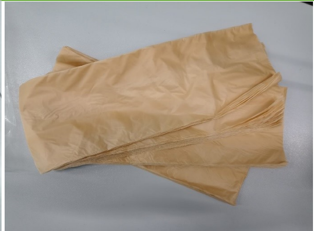
Film blowing of biomaterial by NVMT including lignin at different concentration
