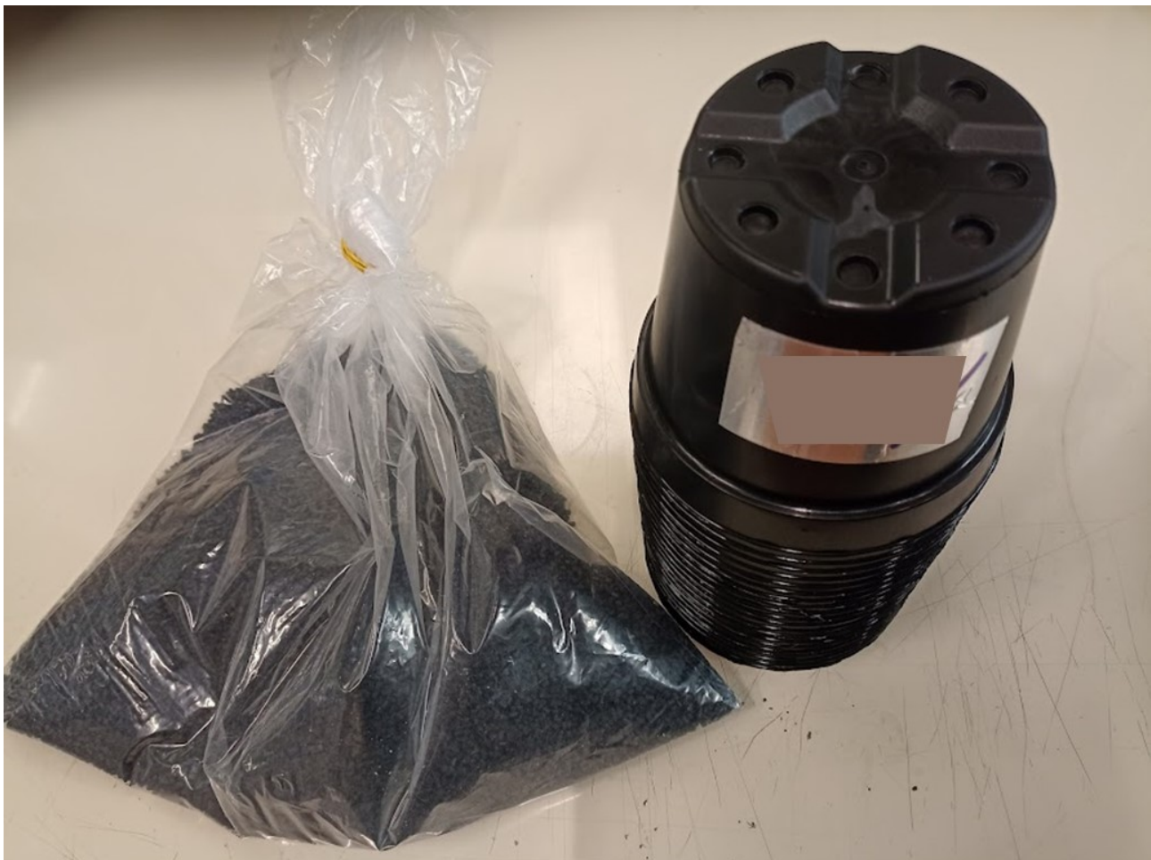
Biomaterial granules and injection molded grow pots obtained by NVMT and including biochar from Miscanthus straw pellet provided by UEDIN.
