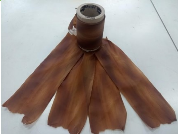
Film blowing of biomaterial by NVMT including lignin at different concentration
