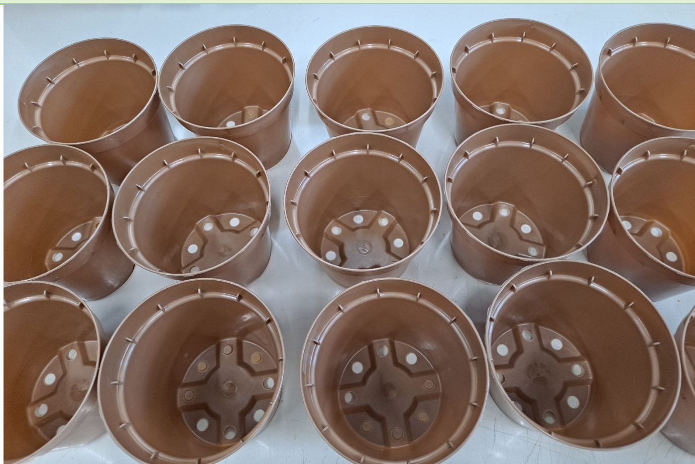
Injection moulded grow pots based on NVMT's biopolyester and including nanolignin
