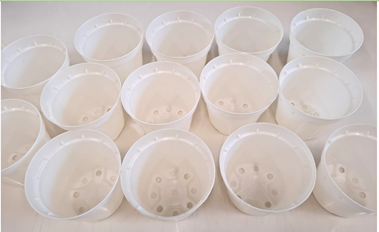
Injection moulded grow pots based on NVMT's biopolyester derived from biobased succinic acid
