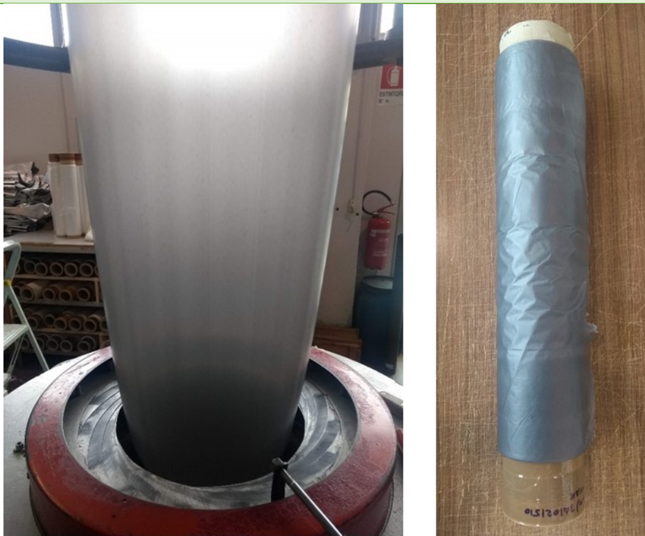
Film blowing of biomaterial by NVMT including biochar and final film roll
